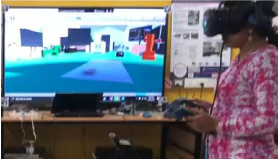
Fusion of Multimodal User Interface with VR for a task involving two users operating sAGV and Cobot simultaneously using non- traditional modalities of interaction
