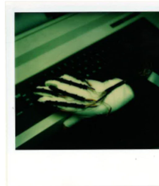
The Sayre glove. The black tubes are the angle transducers which register how much each joint is bent.
