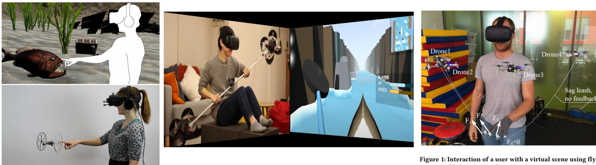
Figure 1. When the user reaches out to touch the virtual anglerfish, our system allows the user to experience a congruent haptic stimulus. Our system controls a quadcopter at the exact location of the virtual fish to provide a synchronized touchable surface.
