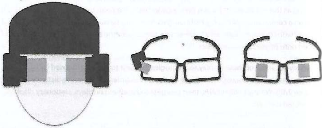
Figure 2.19 Different display mounting options. (left) Helmet-mounted display, like that used by Rockwell Collins SimEye. (middle) Clip-on display, like that used by Google Glass. (right) Visor display, like that used by Epson Moverio.
