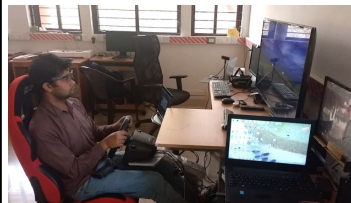
Participant wearing Tobii Glasses and EEG tracker and the Kinect on the table
